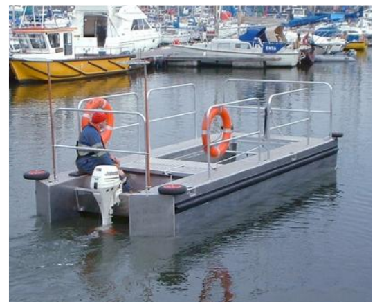
6m Buddy with tiller-controlled 15hp engine
