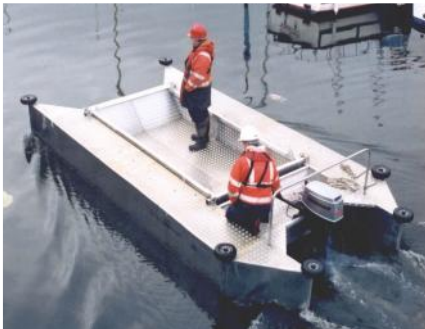
Cargo Pod Designed to carry up to 1 tonne of equipment.
