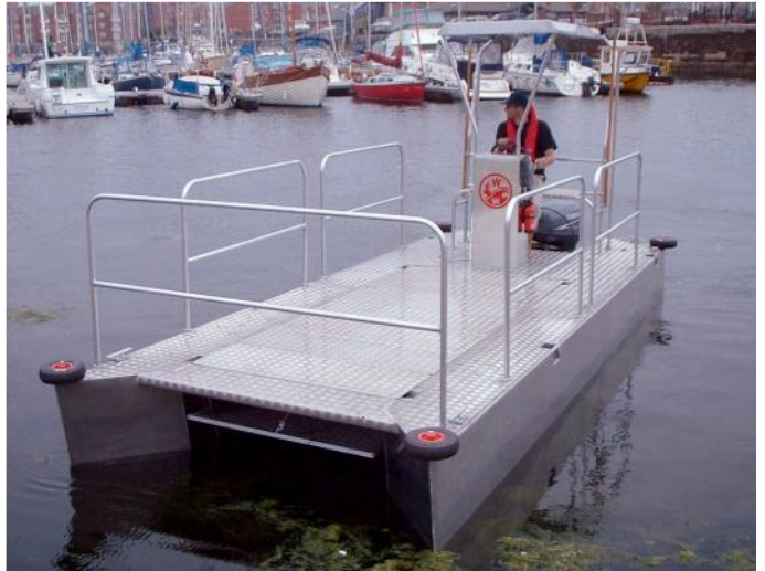
Deck plates provide a 13m 2 working platform
