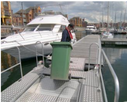
Bow Ramp Heavy-duty loading ramp
