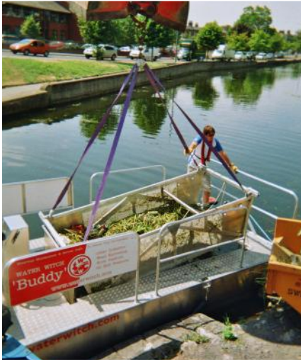
Litter Collection Basket 2.6 cubic meter capacity collection basket with remote-operated front door
