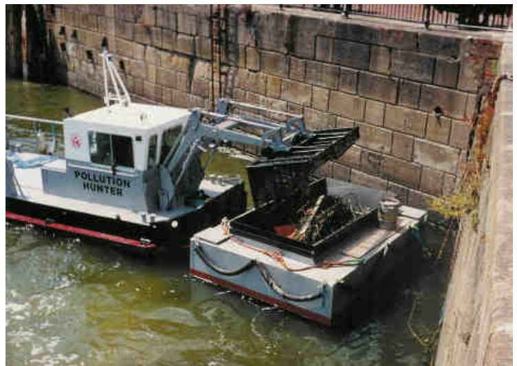
Operating general purpose mesh scoop for efficient removal of large and small items of debris.
